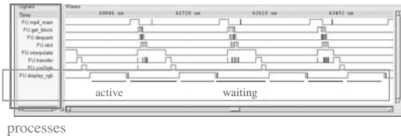
Figure 2. Example of process profiler waveform.
